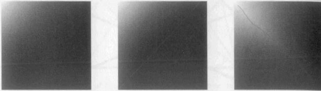
Figure 9.4. The left figure is rendered as a quadrilateral; the middle is two triangles with upper-right and lower-left corners connected; the right shows what happens when the other diagonal is used. The middle figure is better visually than the right one.
