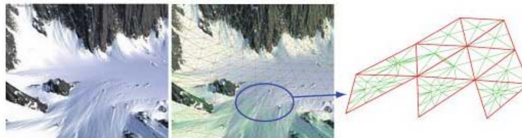
Figure 13.57. Displaced terrain rendering using adaptive fractional tessellation. As can be seen in the zoomed-in mesh to the right, independent fractional tessellation rates are used for the edges of the red triangles, which gives us adaptive tessellation. (Images courtesy of Game Computing Applications Group, Advanced Micro Devices, Inc.)
