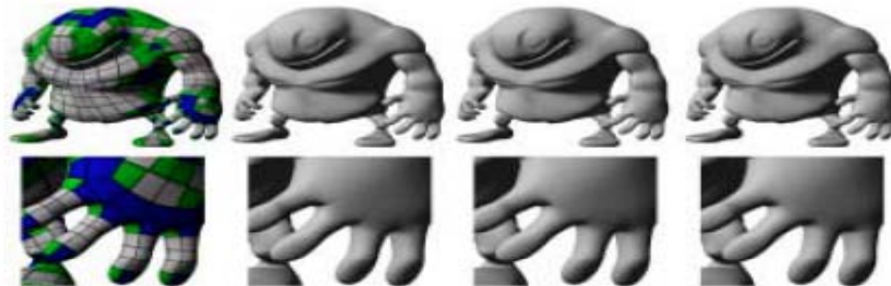
Fig. 10. An example mesh (top) and a zoomed in region of a complex patch structure (bottom). From left to right: Catmull-Clark patch structure, Geometry patch approximation, Geometry/Tangent patch approximation and Catmull-Clark limit mesh.
