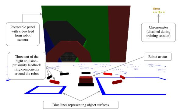
Figure 3: Main Components of the graphical interface.
