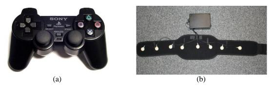
*Figure 4: Interface used in addition to the standard computer monitor: (a) PlayStation 2 dual-shock controller; (b) TactaBelt.*
