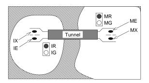
The tunnel controller does not limit the number of cars that it lets through while the light is green. However, the island is small, so a maximum of 16 cars is allowed on the island at any time. The controller has been designed under the assumption that once a car is waiting to use the tunnel, it keeps waiting until it gets to use the tunnel. The desired properties of the controller are as follows:
