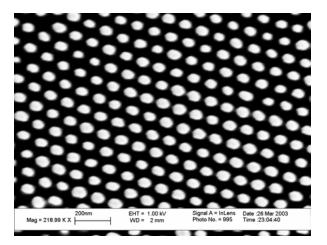
Figure 2: Top view of Si nanopillar array at a different location of the given sample and more zoomed in
