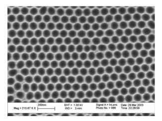
Figure 3: Top view of nanopore array etched into Si
