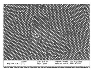
Figure 1: Top view of Si nanopillar array
