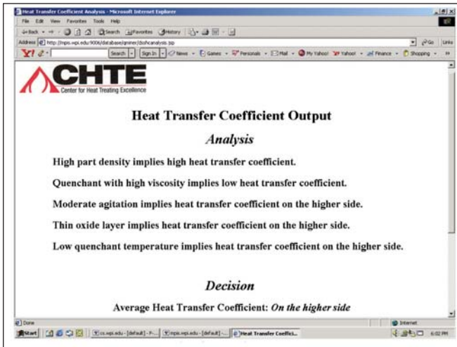
Fig. 3 — Example of QuenchMiner estimation output mation is based on analyzing the results of existing experimental data stored in a database.
