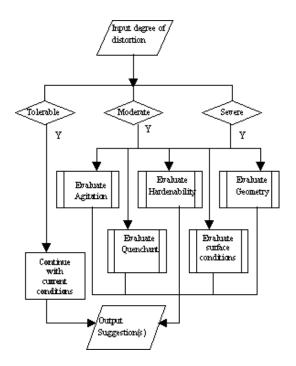
Figure 13: Flowchart for DSS (DistortionCase)
