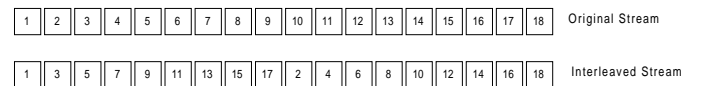
Figure 9: Process of Interleaving frames at the sender (top: original stream, bottom: interleaved stream)
