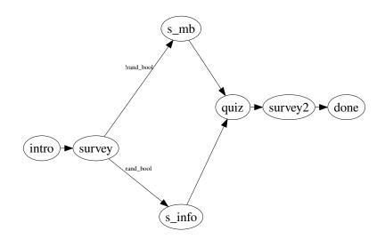
Figure 3.1: State machine for index.cgi
