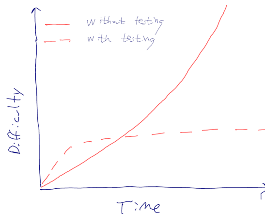
Figure 6.1: The difficulty of code development over time.
