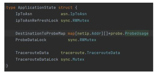
Figure 12: Application State with Each Data Structure Having a Mutex.
