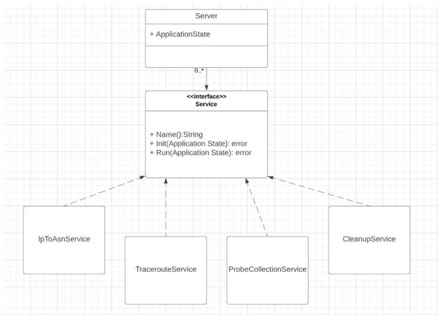
Figure 10: Simplified UML Diagram of the Service Model Used.
