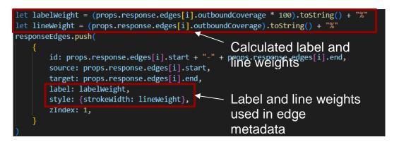
Figure 24: Using outboundCoverage to Determine ReactFlow Edge Weight and Label.
