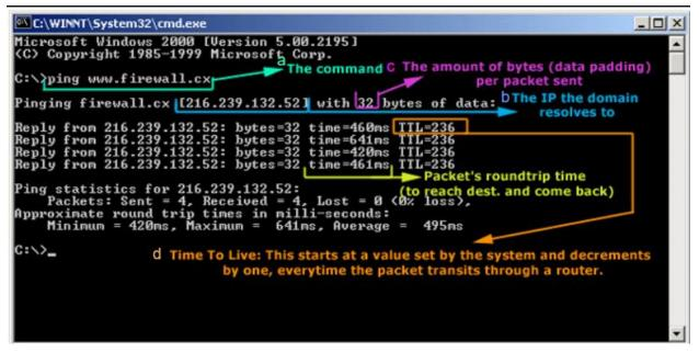
Figure 6: Example Ping Reply.<sup>11</sup>
