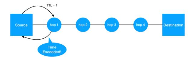
Figure 7: Visualization of Traceroute Hops to the Destination.<sup>16</sup>
