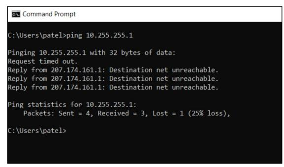
Figure 5: Example of Failed Ping Request.
