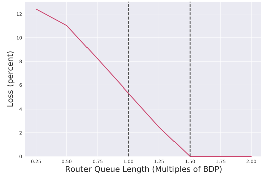
Figure 7. BBR's loss versus router queue size.
