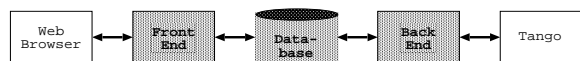
Figure 1: The P-Tango System Architecture. P-Tango consists of a front end, database and back end. The user accesses the front end through a web browser. The back end downloads articles from the Worcester Telegram and Gazette Online (Tango) and makes predictions.
