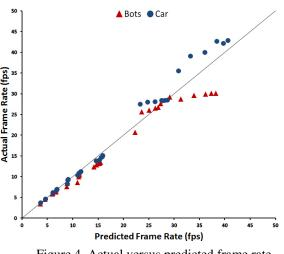
Figure 4. Actual versus predicted frame rate
