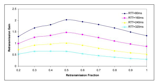
**Figure 7.1.9** Retransmission gain vs. retransmission fraction under different round-trip times for video News (loss rate 10%)
