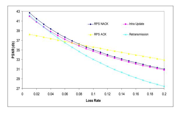
**Figure 7.5.2** PSNR vs. loss for four feedback-based error control techniques (round-trip time=240ms, video News)
