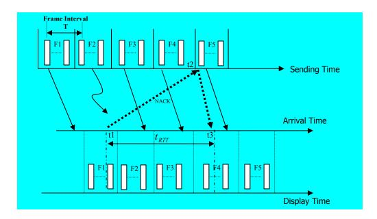
Figure 2.2 Illustration of retransmission scheme
