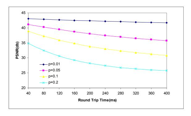
**Figure 7.1.5** PSNR vs. round-trip time with Full Retransmission under different loss rates for video News
