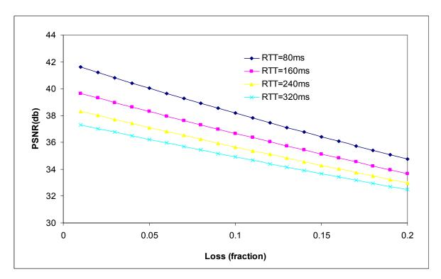
Figure 7.3.3 PSNR vs. loss with RPS ACK under different round-trip times (video News)
