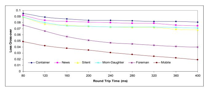
**Figure 7.5.11** The loss crossover point for loss vs. round-trip time for six video clips using PSNR
