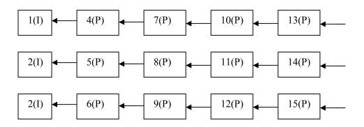
Figure 6.6 RPS ACK, round-trip time = 3 frames, frame 3 and 4 are lost
