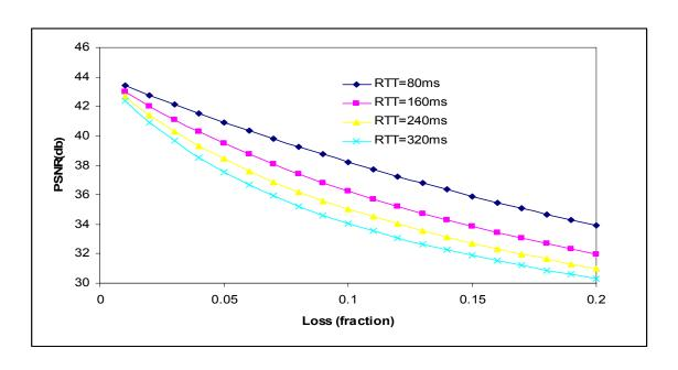
**Figure 7.2.3** PSNR vs. loss with RPS NACK under different round-trip times (video News)
