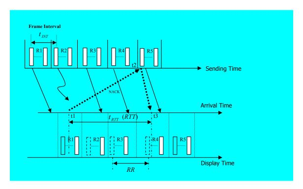
**Figure 4.1** Illustration of Retransmission Range (RR), where each rectangle represents a GOB, and the rectangle with dashed-line indicates the GOB is either lost or cannot be decoded correctly due to error propagation.
