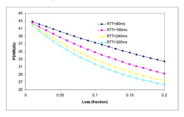
**Figure 7.1.3** PSNR vs. loss with Full Retransmission under different round-trip Times for video News
