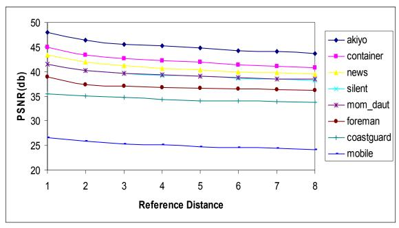
**Figure 5.2** PSNR vs. reference distance for video clips with different content characteristics
