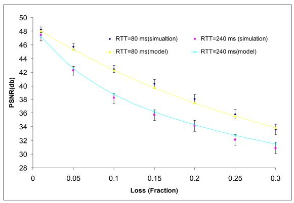
Figure 6.7 PSNR vs. loss with RPS NACK (video clip: Akiyo)
