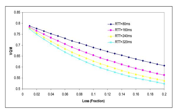
**Figure 7.1.4** VQM vs. loss with Full Retransmission under different round-Trip Times for video News
