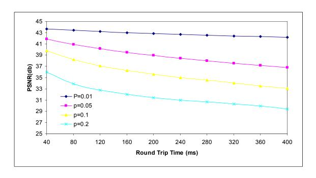
**Figure 7.2.1** PSNR vs. round-trip time with RPS NACK under different loss rates (video News)
