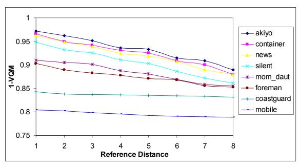
Figure 5.4. VQM vs. reference distance for video clips with different content
