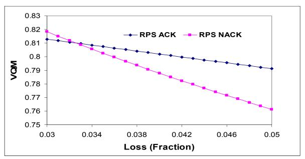
Figure 7.5.8 RPS NACK vs. RPS ACK (round-trip time = 400 ms)
