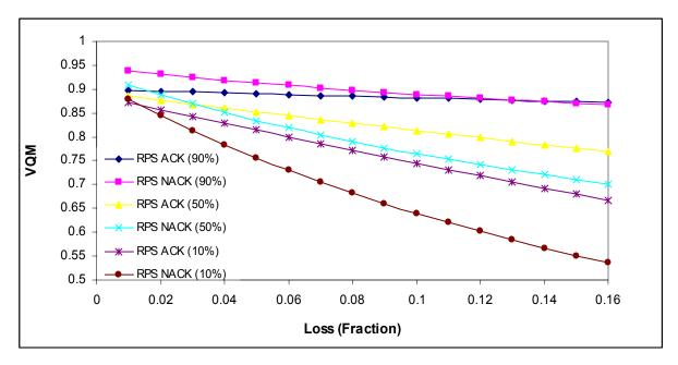
Figure 7.5.9 RPS ACK vs. RPS NACK by varying quality for locally concealed GOBs
