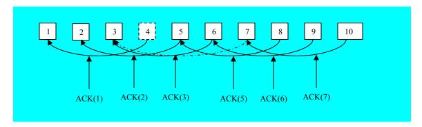
**Figure 2.3.** Illustration of the encoding of GOBs using RPS with ACK mode, where GOB 4 has a transmission error and the arrows indicate the selected reference pictures.
