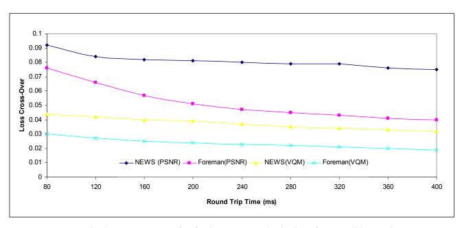
Figure 7.5.12 The loss crossover point for loss vs. round-trip time for two videos using both PSNR and VQM
