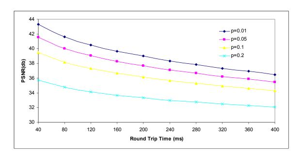
**Figure 7.3.1** PSNR vs. round-trip time with RPS ACK under different loss rates (video News)
