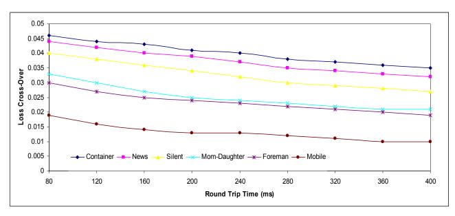
**Figure 7.5.10** The loss crossover point for loss vs. round-trip time for six video clips using VQM
