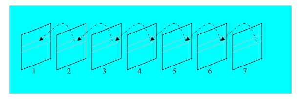
**Figure 4.0** Illustration of a reference chain, where each rectangle represents a video frame, the area between two lines in each rectangle represents a group of macroblocks (GOB), and the arrows indicate the selections of reference-GOB.
