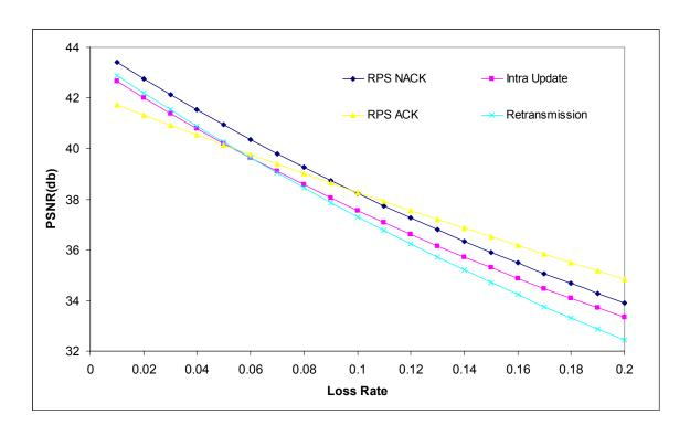
**Figure 7.5.1** PSNR vs. loss for four feedback-based error control techniques (round-trip time=80ms, video News)
