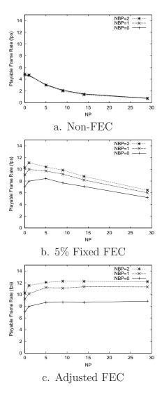
Figure 4.4: Streaming *Foreman* with FEC and PETS. Network model has 2% loss and 1.5 Mbps capacity constraint
