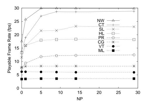
Figure 4.5: Streaming the other 8 videos with adjusted FEC and PETS, 2% loss and 1.5 Mbps capacity constraint  $(N_{BP} = 2)$ .
