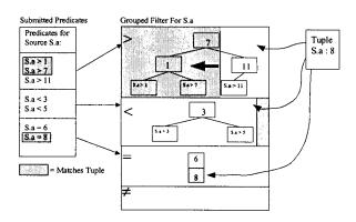
Figure 5: Grouped Filter Example: The grouped filter is searched for matching predicates when a tuple arrives. The grayed regions correspond to matching predicates for the tuple in the upper right.
