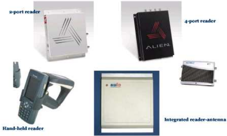
Figure 2: RFID tag readers
