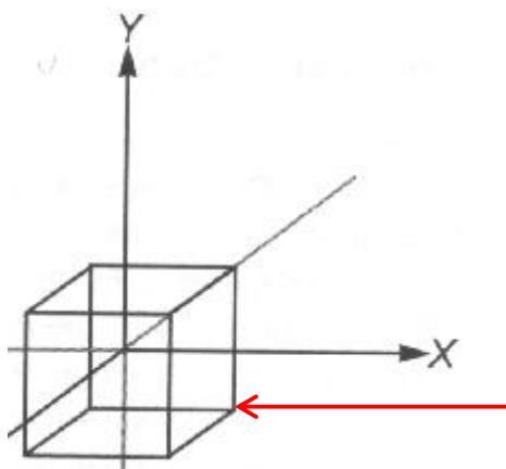
Each vertex of cube is multiplied by modelview matrix to get scaled vertex position
