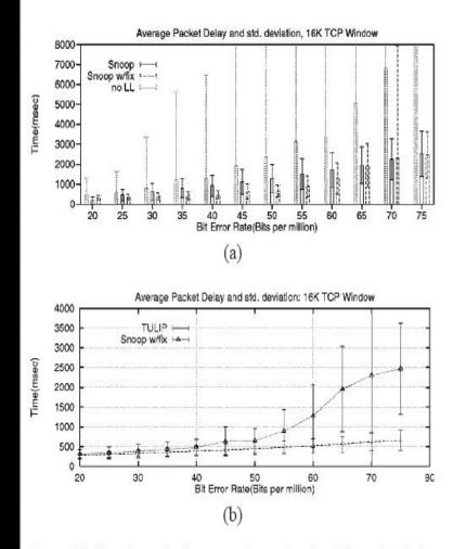
Figure 17. Experiment 2: Average end-to-end packet delay and std. deviation with high error rates and 16 Kbyte receiver window. (a) Snoop, Snoop w/fix and no LL, (b) Snoop w/fix and TULIP.
