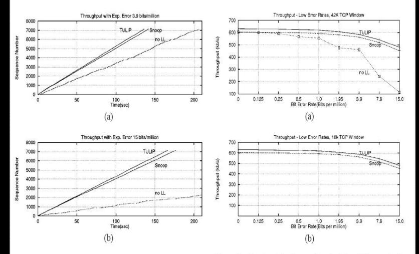
Figure 9. Experiment 1: TCP Sequence number growth. (a) BER = 3.9 bits/million = 1/256 Kbytes, (b) BER = 15 bits/million = 1/64 Kbytes. Receiver window 42 Kbytes.
