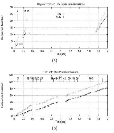
Figure 12. Experiment 1: Sequence number and ACKs at the source for the first 2 seconds of the TCP transfer. Packets dropped on the channel are shown with arrows. BER = 15 bits per million. (a) No link retransmissions, (b) TULIP protocol.
