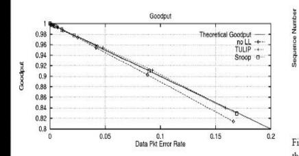
Figure 11. Experiment 1: Goodput for all three protocols with varying packet error rates and a receiver window of 42 Kbytes.
