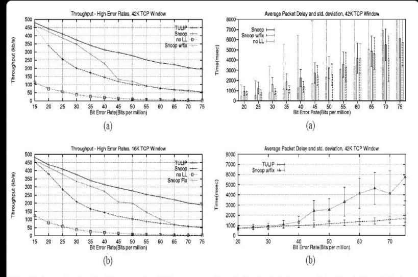
Figure 15. Average throughput for all three protocols with high error rates. (a) 42 Kbyte window, (b) 16 Kbyte window.
