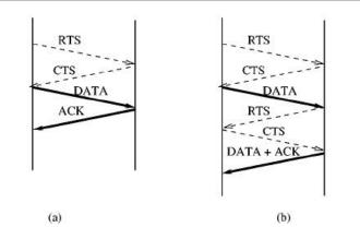
Figure 4. (a) *MAC Acceleration:* FAMA transmits TULIP data packet and returns ACK without another RTS/CTS exchange. Returning TULIP ACK may contain a TCP ACK. (b) FAMA exchange with large ACK packet (encapsulated data packet) requires another RTS/CTS exchange.
