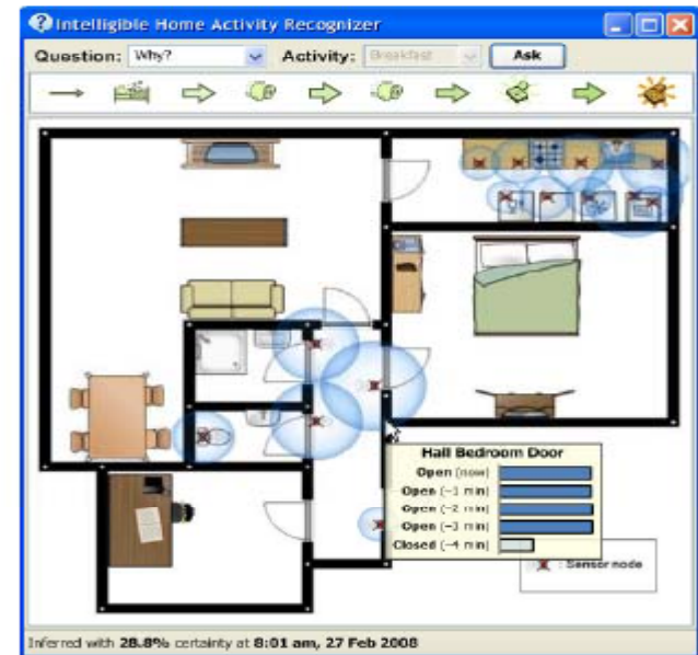
Figure 8: Demonstration of Why explanation visualization from an application using a HMM to model domestic activity.
