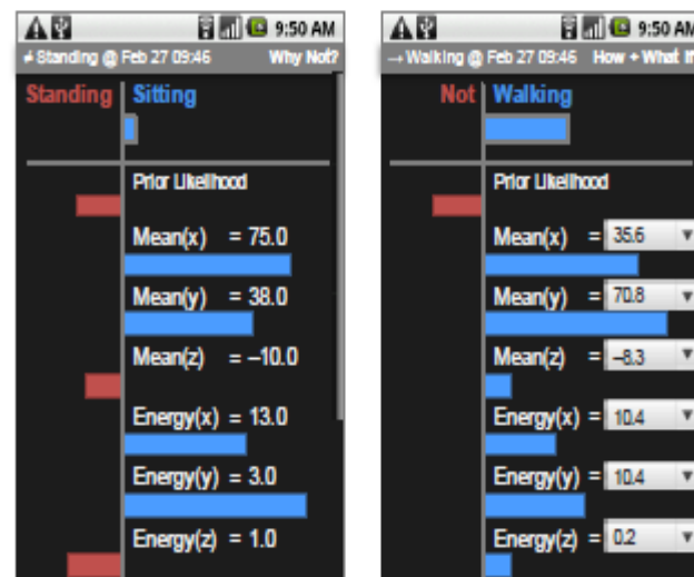
Figure 6: Why Not (Left), and How To + What If (Right) explanations for a mobile phone physical activity recognition application using accelerometer data trained with a naïve Bayes classifier. The application has inferred that the user is Sitting .
