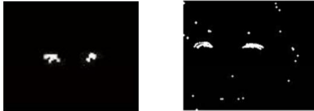
Figure 1: Left figure: example of eye contour pair returned by the original algorithm running on a desktop with a USB camera. The two white clusters identify the eye pair. Right figure: example of number of contours returned by EyePhone on the Nokia N810. The smaller dots are erroneously interpreted as eye contours.
