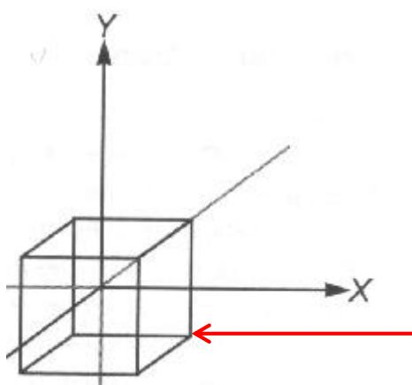
Each vertex of cube is multiplied by modelview matrix to get scaled vertex position
