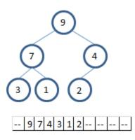
Note in the array representation you lose the 0<sup>th</sup> element, so it is shown as a --. Then the heap is constructed with 11 total spaces, the last four of which are unused. Finally you read off the heap left to right by level.
