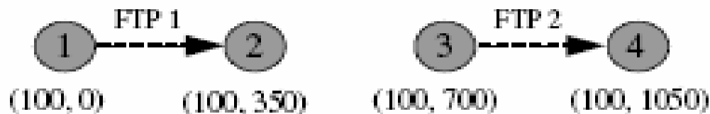
Figure 8: The hidden terminal scenario, where Node 2 is hidden by transmission from node 4 to node 3 and Node 3 is hidden by transmission from node 1 to node 2.
