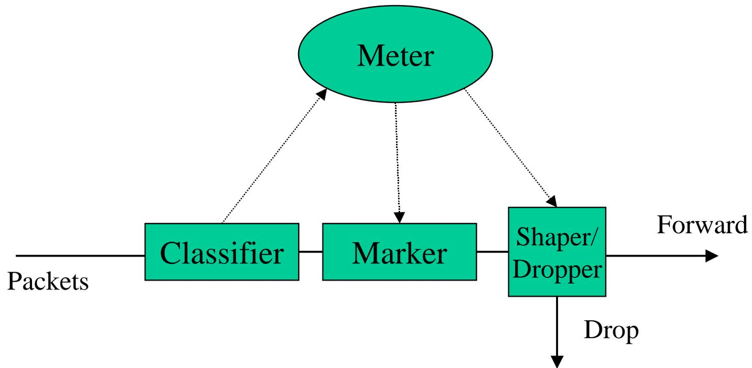
Logical view of packet classification and traffic conditioning at the edge router
