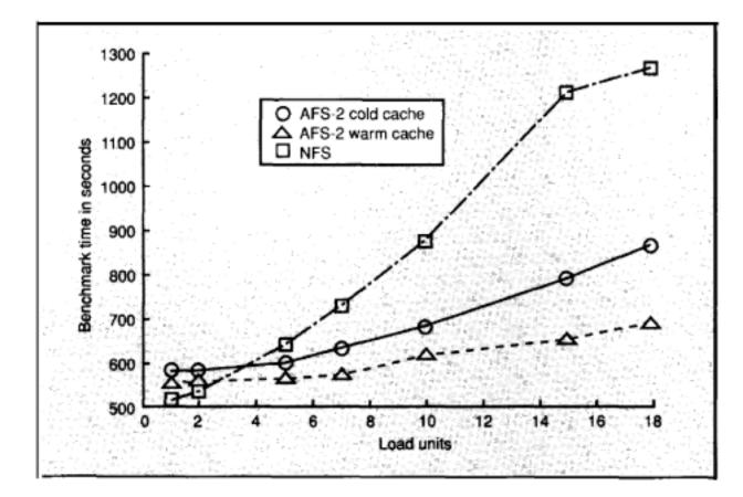
Load unit consists of one client workstation running an instance of the Andrew benchmark.
