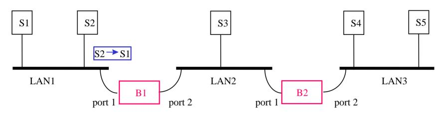
Bridge 1 does not forward the frame to LAN2
