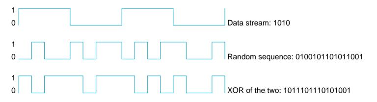
Figure 2.37 Example 4-bit chipping sequence
