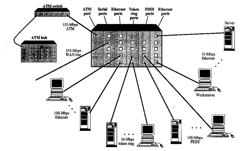
Figure 5.10 ATM LAN hub configuration.
