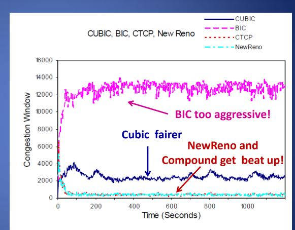
Fig. 2. Congestion window curves for CUBIC, BIC, CTCP and NewReno flows. A congestion window curve represents the sum of 20 flows of a type [Munif 2007]
