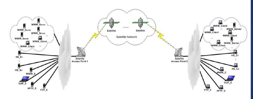
Fig. 1. Network Topology: Two High Speed Networks Connected Through Satellite Network
