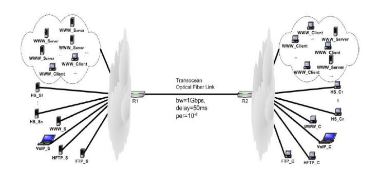
Figure 1: Wide Area Network Scenario: High Speed Congestion Control Algorithms on a Transocean Optical Fiber Link
