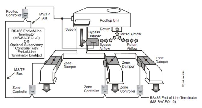
Figure 1: Typical Zoning Control System Installed on a Single MS/TP Bus
