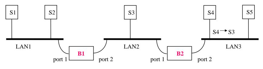
Bridge 1 does not forward the frame to LAN1
