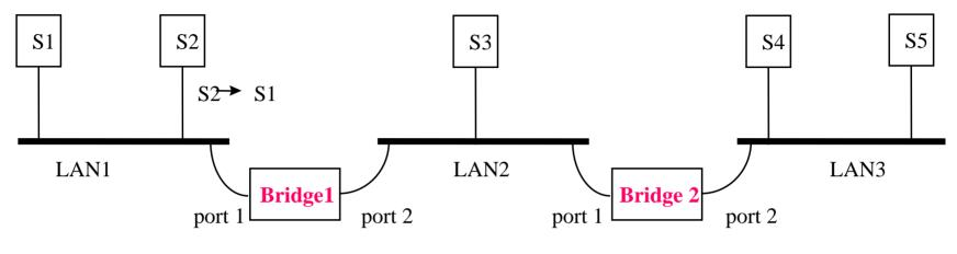
Bridge 1 does not forward the frame to LAN2
