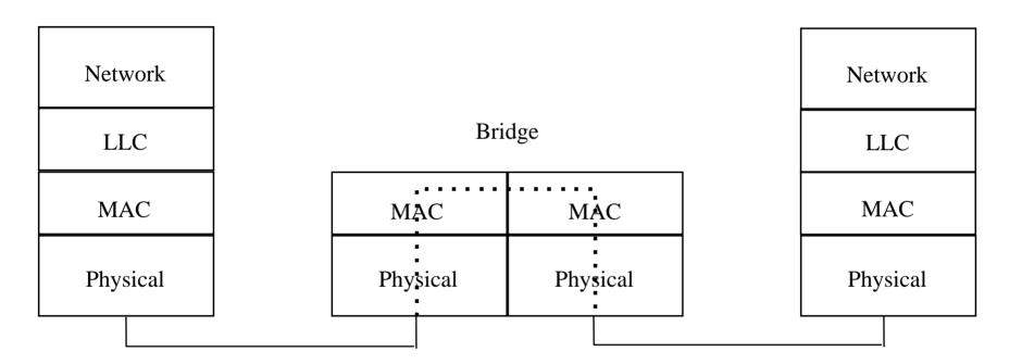
A bridge is a store and forward device that **separates** collision domains.
