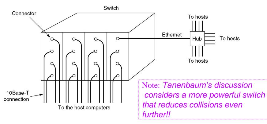
Figure 4-20.A simple example of switched Ethernet.
