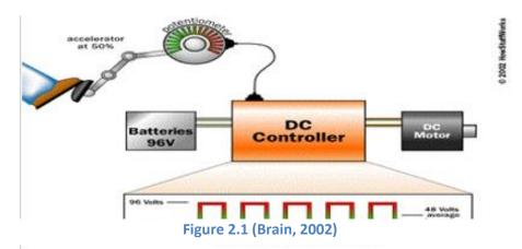
Figure 2.1 shows how a DC controller in an EV functions. The DC controller is connected to the battery pack and DC motor. When the driver pushes on the pedal the controller determines the amount of voltage transferred from the battery to the motor which dictates the speed of the car.
