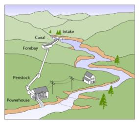
Figure 2.10: Typical Construction of a Run of the River Hydroelectric Power System (Department of Energy, 2009)
