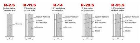
Figure 2.3: Effects of Adding Insulating Materials to the R-Value of a Concrete Wall (McMichael, 2010)
