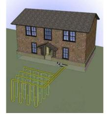
Figure 2.14: Schematic of Curry Village Ground Source Heat Recovery System (National Park Service 2010)
