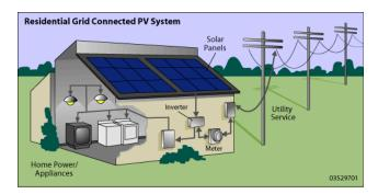
Figure 2.5: Grid Connected Photovoltaic System (Department of Energy, 2009)
