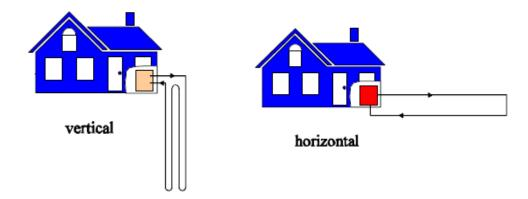
Figure 2.12(a): Vertical Closed LoopFigure 2.12(b): Horizontal Closed Loop(Lund, J. Sanner, B. Rybach, L. Curtis, R. Hellstrom, G. 2004)
