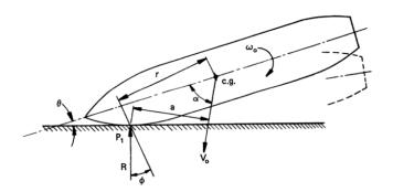
Figure 9. Visual reference for berthing energy calculations. (Gaythwaite, 2004)
