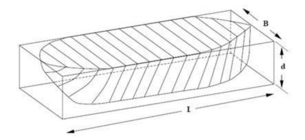
Figure 10. Visual reference for block coefficient calculations. (Transport Canada, 2010)
