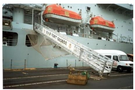
Figure 14. A typical ship gangway. (Clow Group Ltd., 2011)
