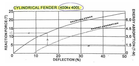
Figure 11. Visual reference for berthing force calculation. (Wang, 2009)
