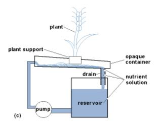
Figure 2-4: Nutrient Film Technique Source: Dreschel, 2014
