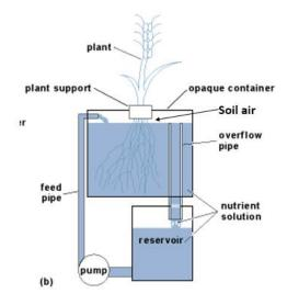
Figure 2-5: Dynamic Root Floating Technique Source: Dreschel, 2014
