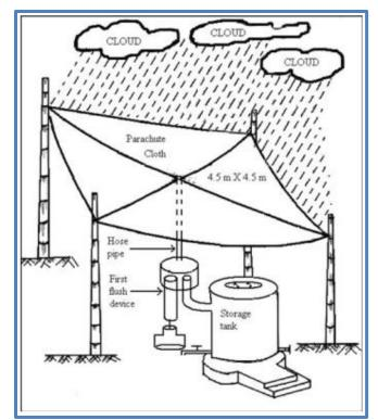
Figure 2-4: Schematic Drawing of the Rainwater Harvesting System in Dhaka, Bangladesh (M. M. Islam et al., 2010)
