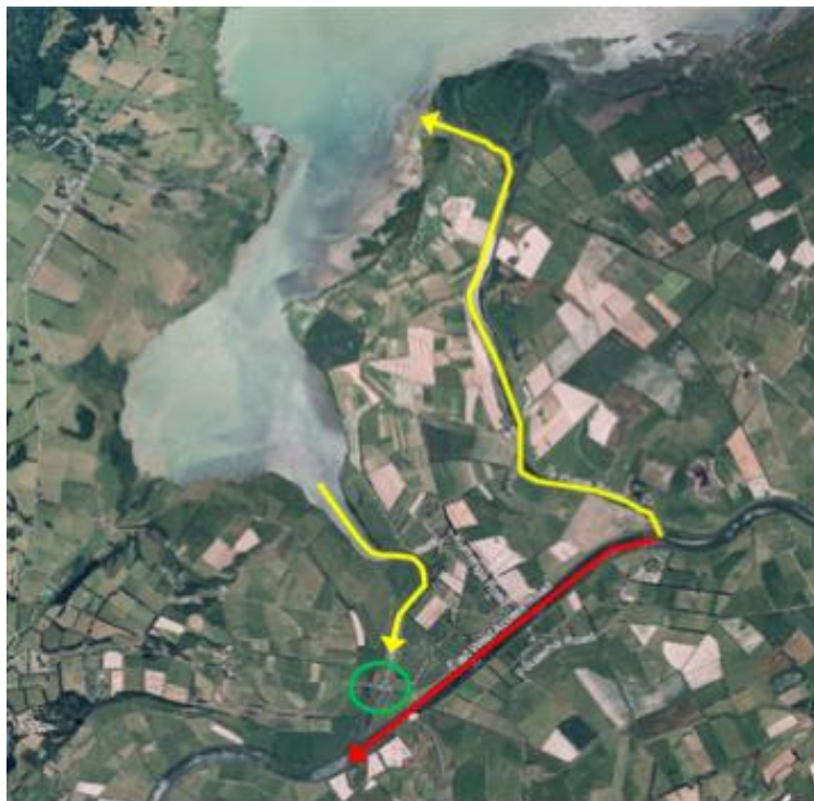
Figure 7: Yellow lines show the previous, natural path of the Ruamahanga River. The red line shows the Ruamahanga Diversion and the current path of the river. The green circle show the location of the barrage gates. (Google, 2015)
