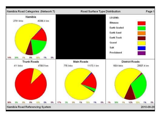
Figure 15: Road surface type distribution of various road surfaces in Namibia by road location (Roads Authority, 2011)
