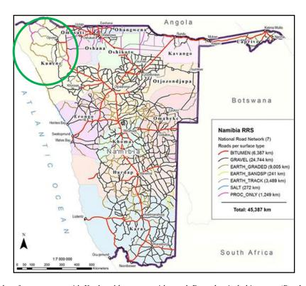
Figure 16: Road surface type map with Kaokoveld, an area with rough D roads, circled in green (Roads Authority, 2011)
