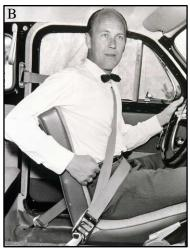
Figure 7: (left) A. Young woman fastening a two-point safety belt, circa 1950 (pinterest.com) (right) B. Nils Bohlin, inventor of the three-point safety belt, demonstrating its use in 1959 (wired.com)
