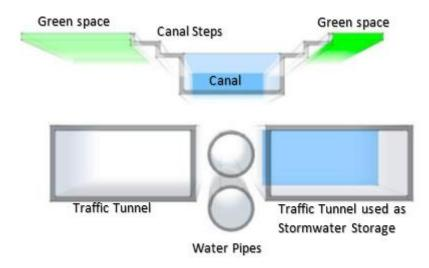
FIGURE 44: APPENDIX D CROSS SECTION OF PROPOSED TUNNEL DESIGN (RUDDY ET AL., 2012)
