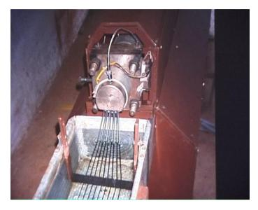
Figure 14: Example of Pelletizer Machine in India (Van Den Berg, 2009)
