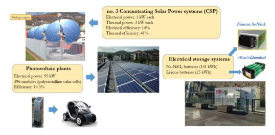
Figure 3: Smart Polygeneration Microgrid at Genoa University (Brenna et al., 2016).
