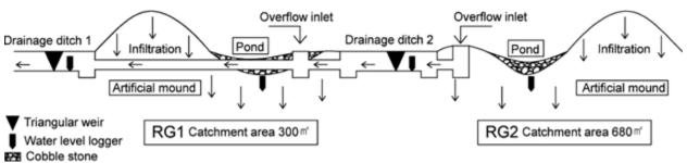
Figure 2.18: Diagram of the rain garden designs used in the Kyoto Prefecture study (Zhang et al., 2020)
