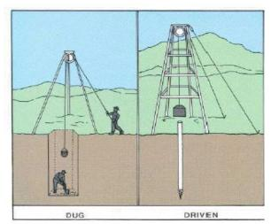
Figure 2.16: Dug wells versus driven wells (Waller, 2016.)
