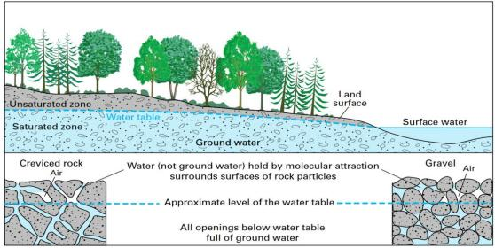
Figure 2.15: Description of water table and water saturation of the area below the water table (USGS, n.d.)
