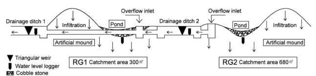
Figure 2.11: Diagram of the rain garden designs used in the Kyoto Prefecture study (Zhang et al., 2020)
