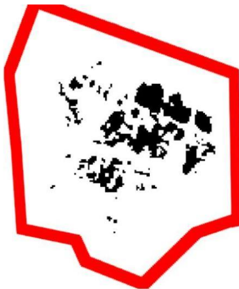
Figure 2.12. VNP Water body extraction in GIS software using NDWI
