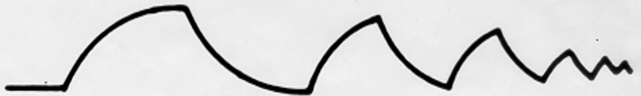
FIGURE 2.1 Attenuation of Digital Signals
