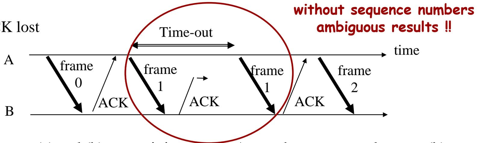
In parts (a) and (b) transmitting station A acts the same way, but part (b) receiving station B accepts frame 1 twice.
