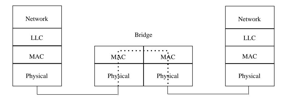
A bridge is a store and forward device that <u>separates</u> collision domains.
